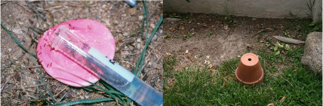
**Figure 2.** Styrofoam dam and pipette used for water sampling.
