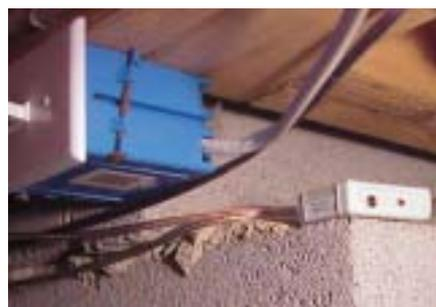
*Electronic monitoring near joist in test crawl.*
